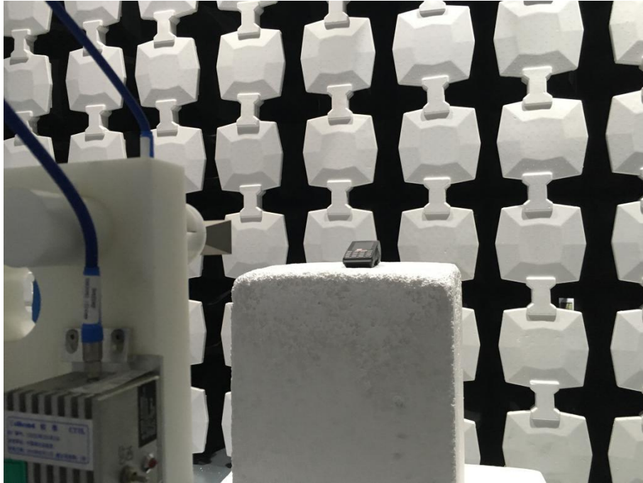
Description: Radiated Emission Test Setup (Above 18GHz)
