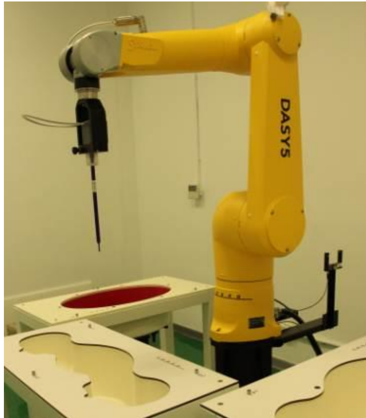
Picture D.6 DSY5 system Set-up
