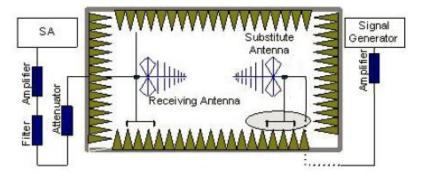
In the chamber, an substitution antenna for the frequency band of interest is placed at
