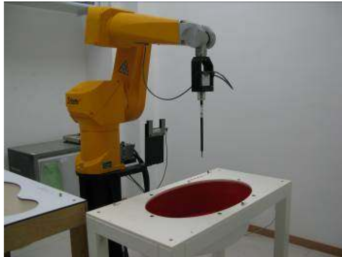
Fig.A-1 Photograph of the SAR measurement System
