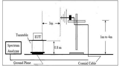
(B) Radiated emission Test setup frequency over 1GHz:
