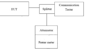
Measurement Setup for testing on Antenna connector.
