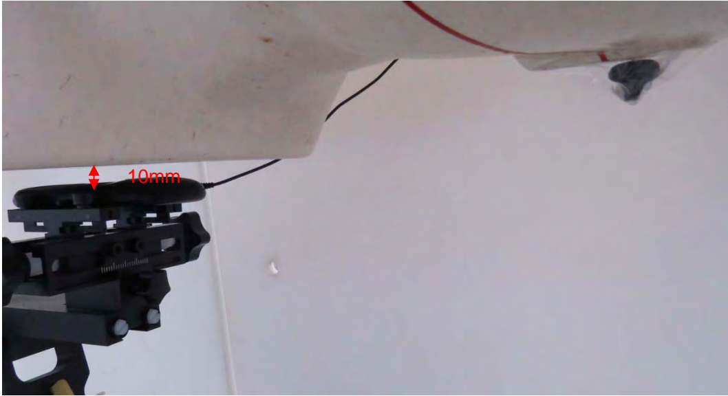
Picture 14: Back Side with Earphone, the distance from handset to the bottom of the Phantom is 10mm
