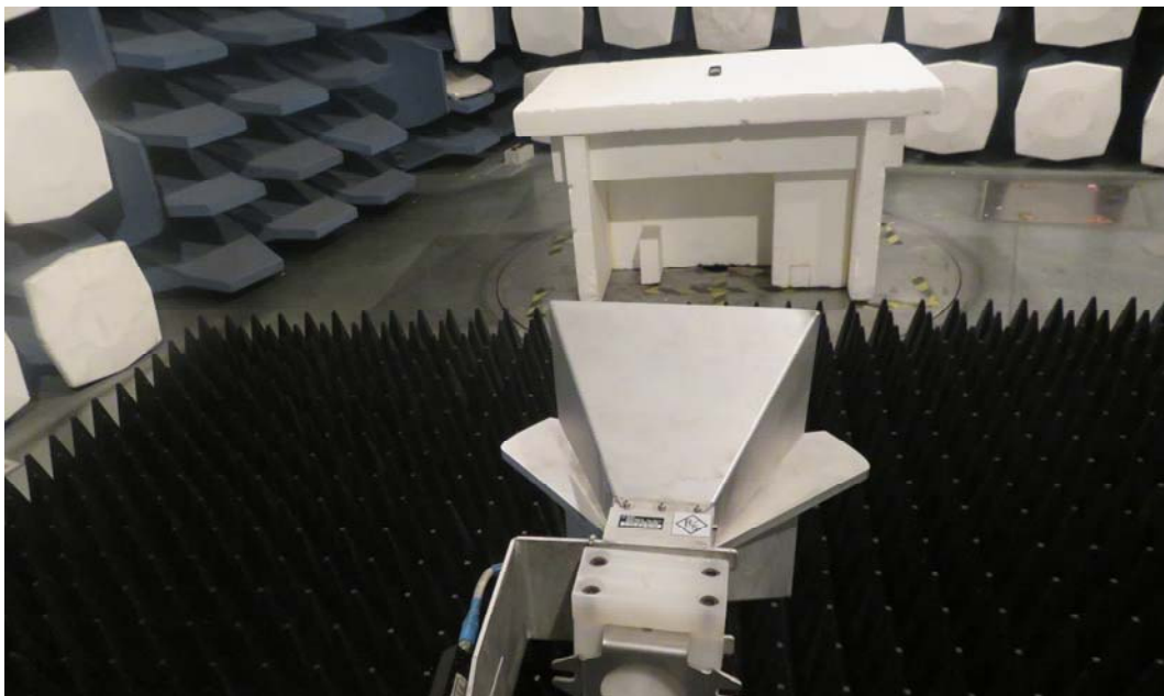
Picture 2: Radiated Spurious Emissions Test setup
