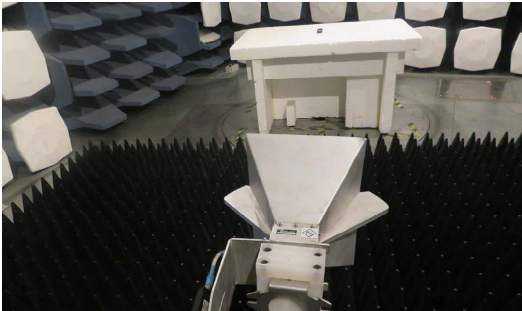
Picture 2: Radiated Spurious Emissions Test setup
