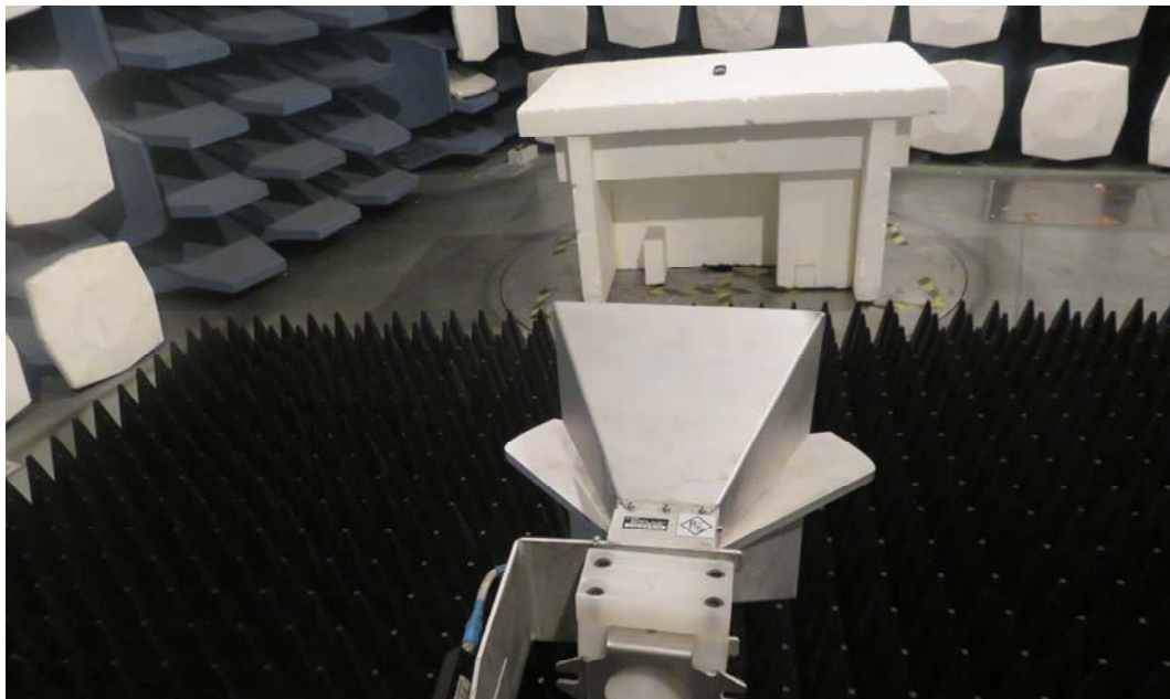
Picture 2: Radiated Spurious Emissions Test setup
