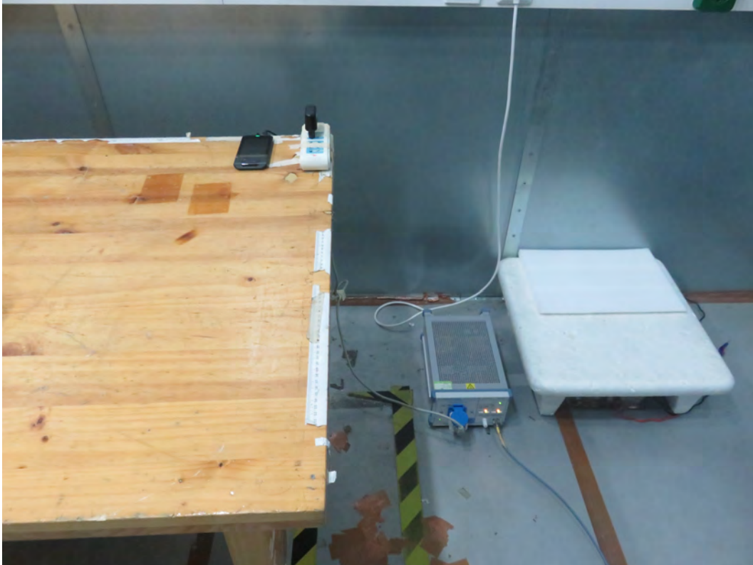
Picture 3 Conducted Emission Test Setup
