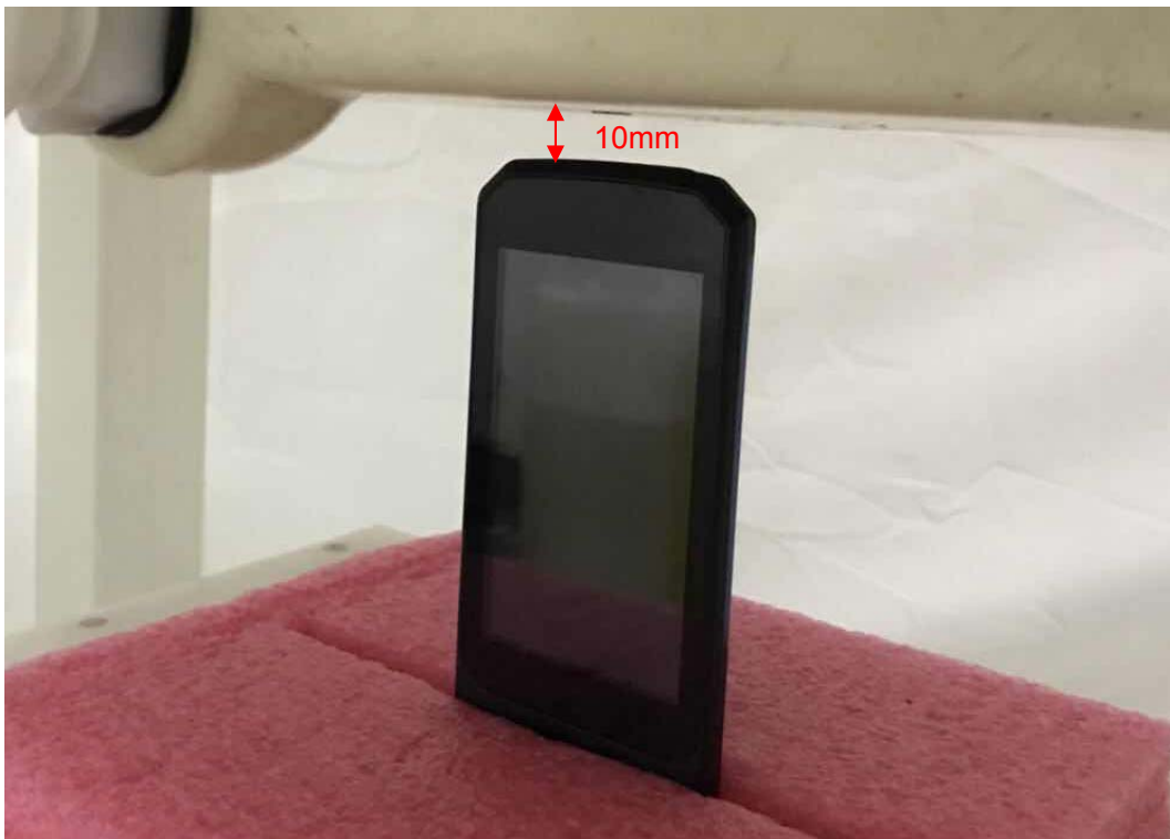
Picture 10: Bottom Side, the distance from handset to the bottom of the Phantom is 10mm
