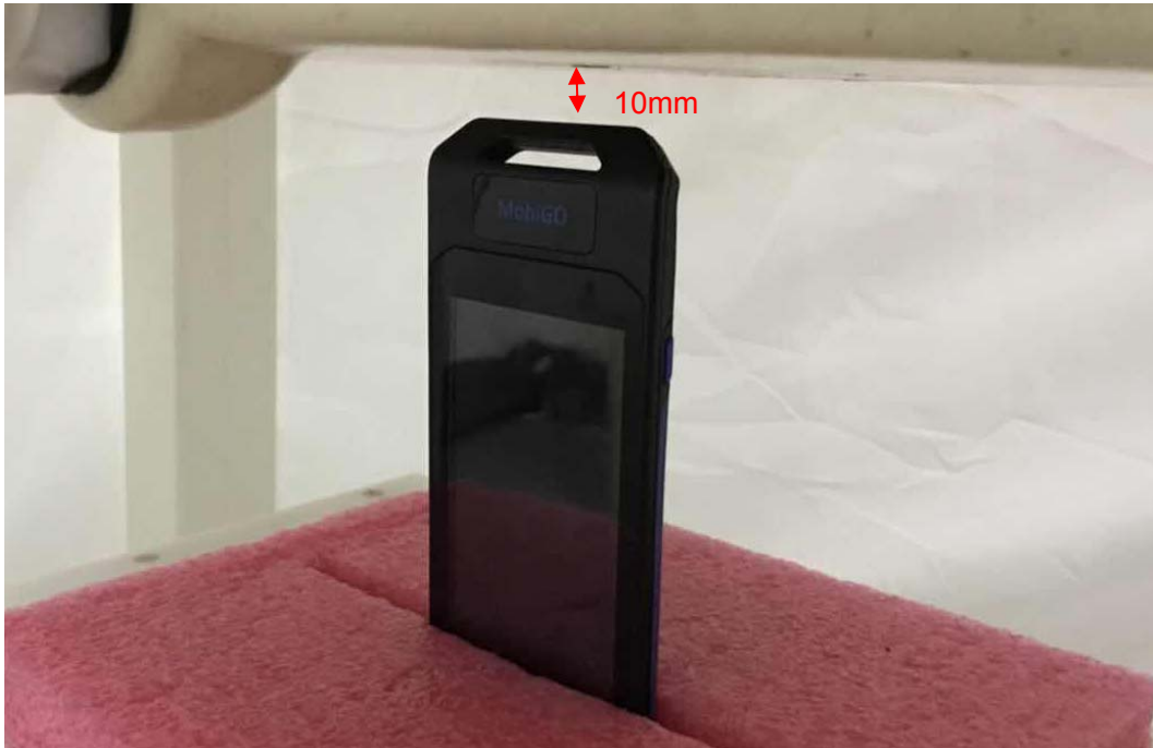
Picture 9: Top Side, the distance from handset to the bottom of the Phantom is 10mm
