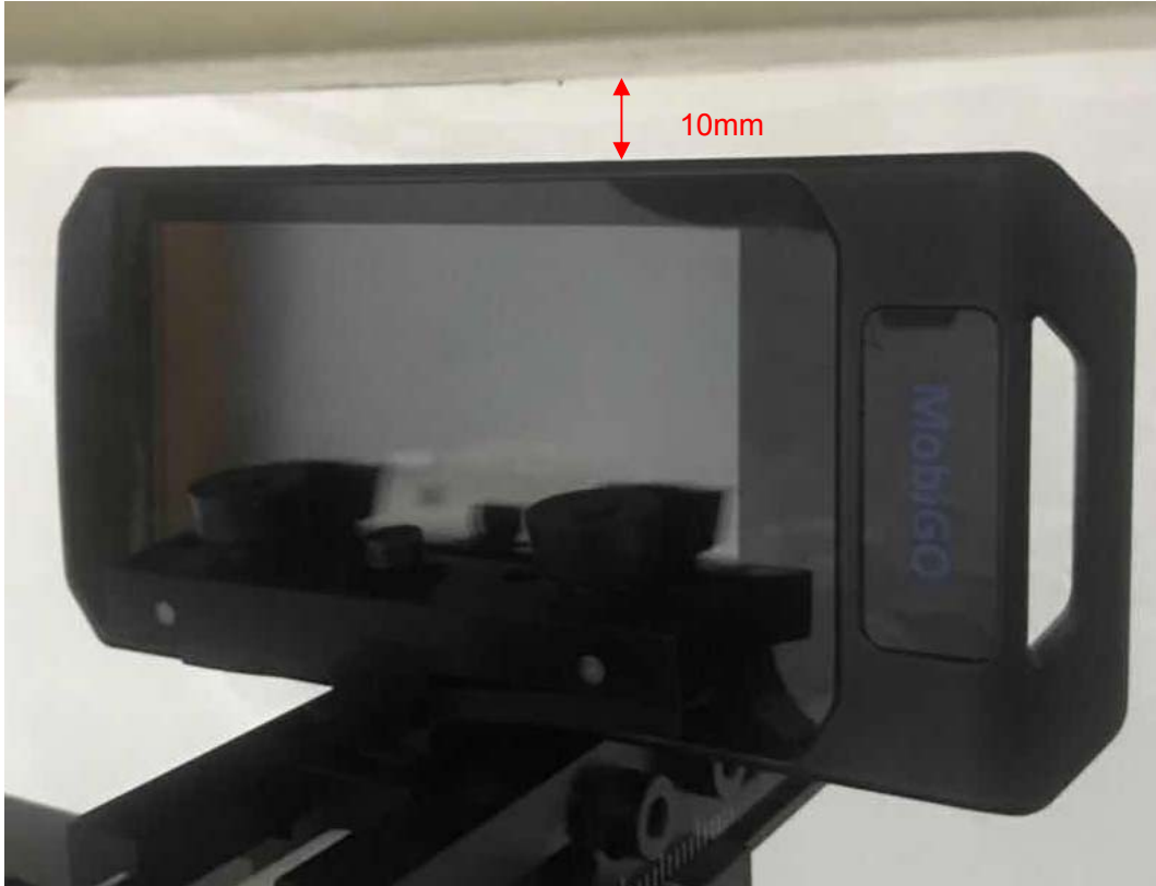
Picture 7: Left Side, the distance from handset to the bottom of the Phantom is 10mm
