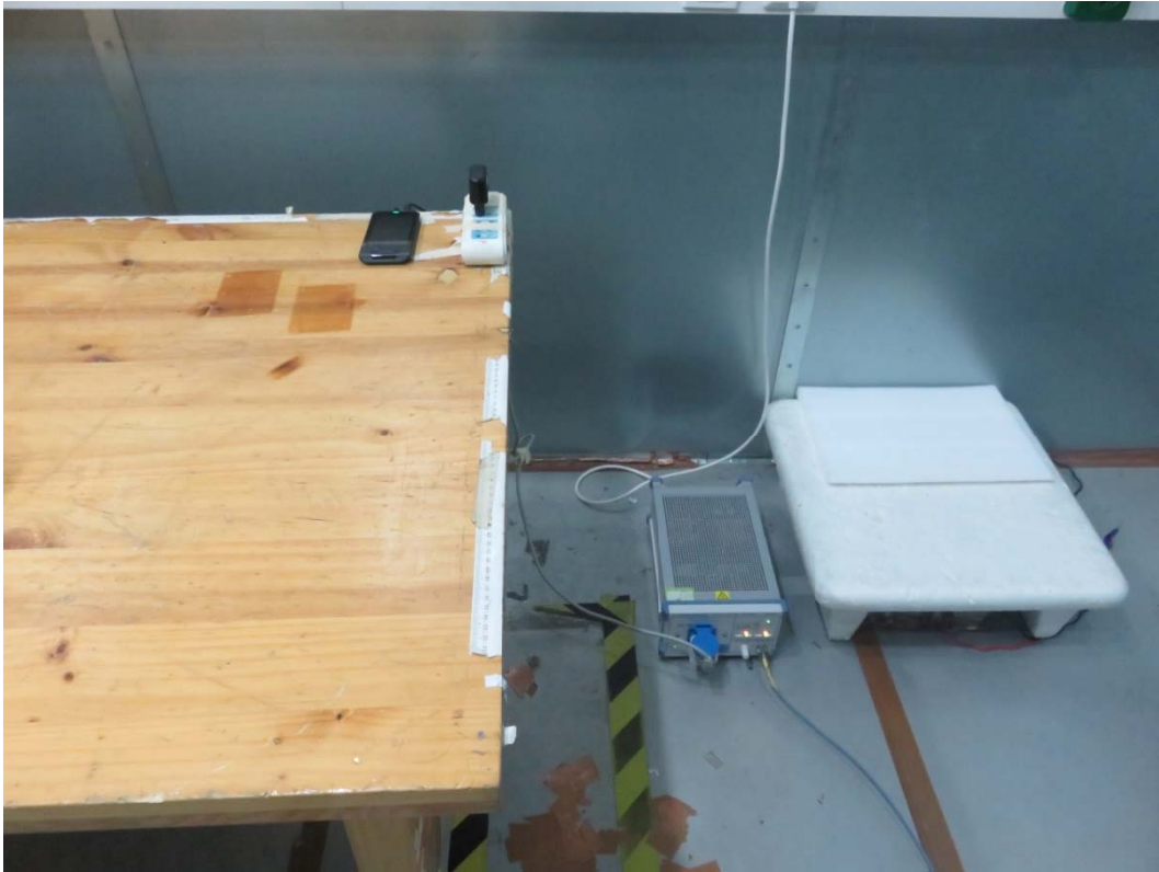
Picture 3 Conducted Emission Test Setup
