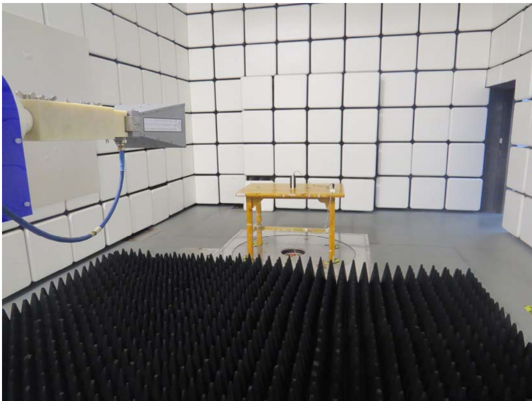
Picture 2: Radiated Spurious Emissions Test setup
