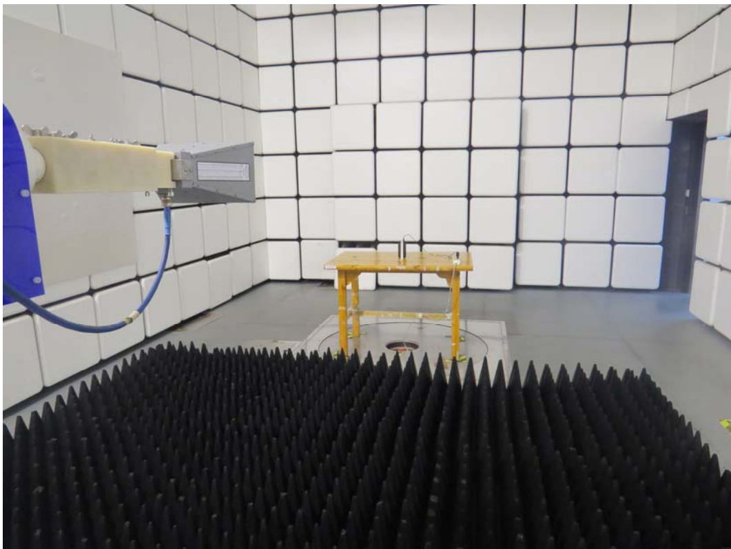
Picture 2: Radiated Spurious Emissions Test setup
