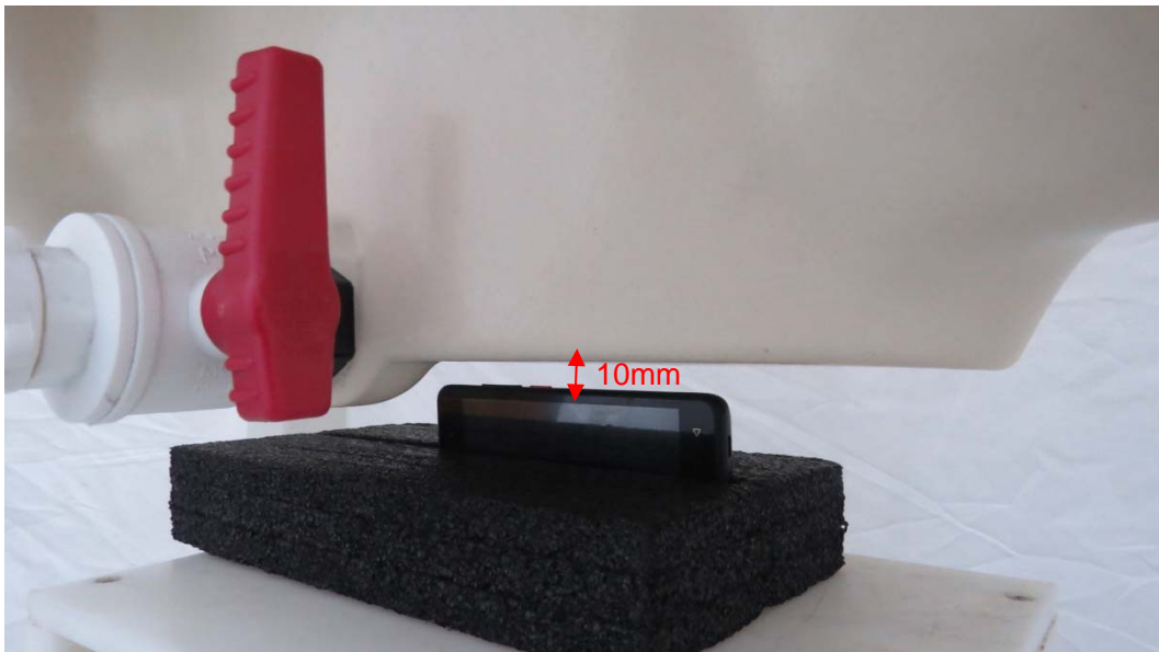
Picture 8: Right Side, the distance from handset to the bottom of the Phantom is 10mm
