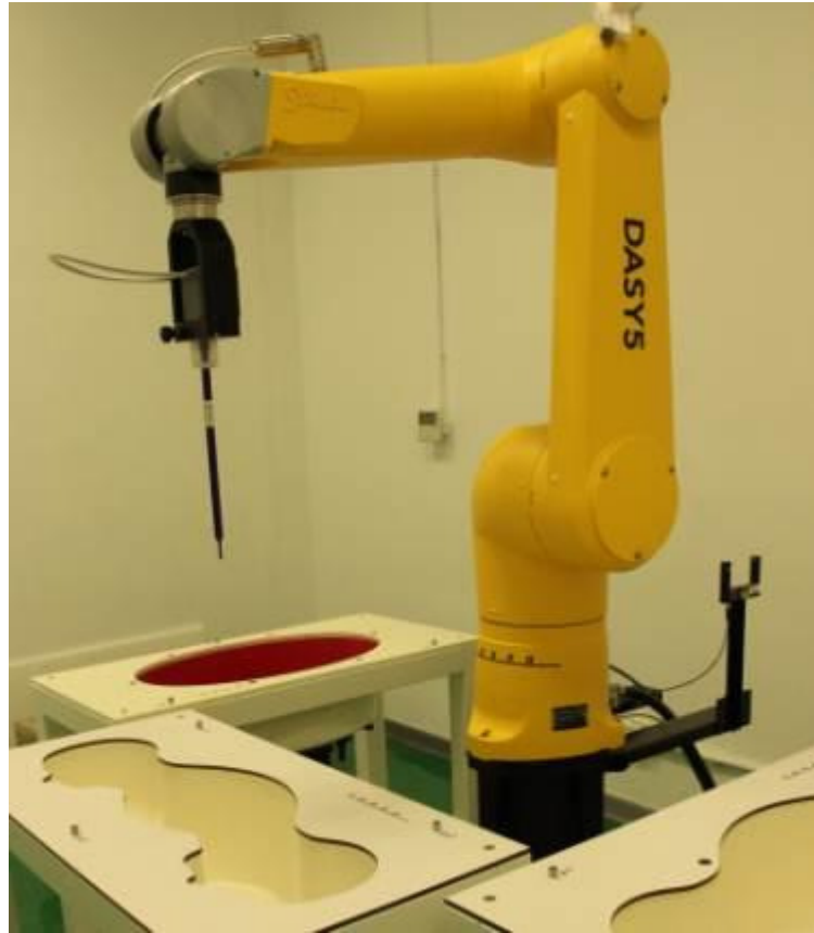
Picture D.6 DSY5 system Set-up
