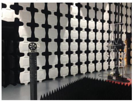
Description: Substitution Antenna for ERP Test
