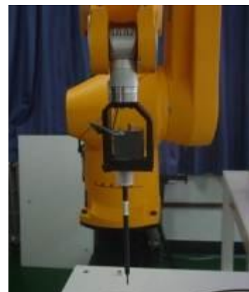
Picture C.3 E-field Probe
