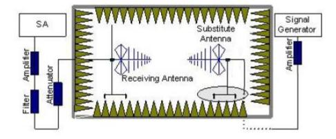
In the chamber, a substitution antenna for the frequency band of interest is placed at the reference
