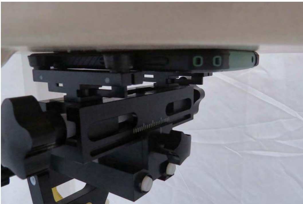
Picture 19: Front Side, the distance from handset to the bottom of the Phantom is 0mm
