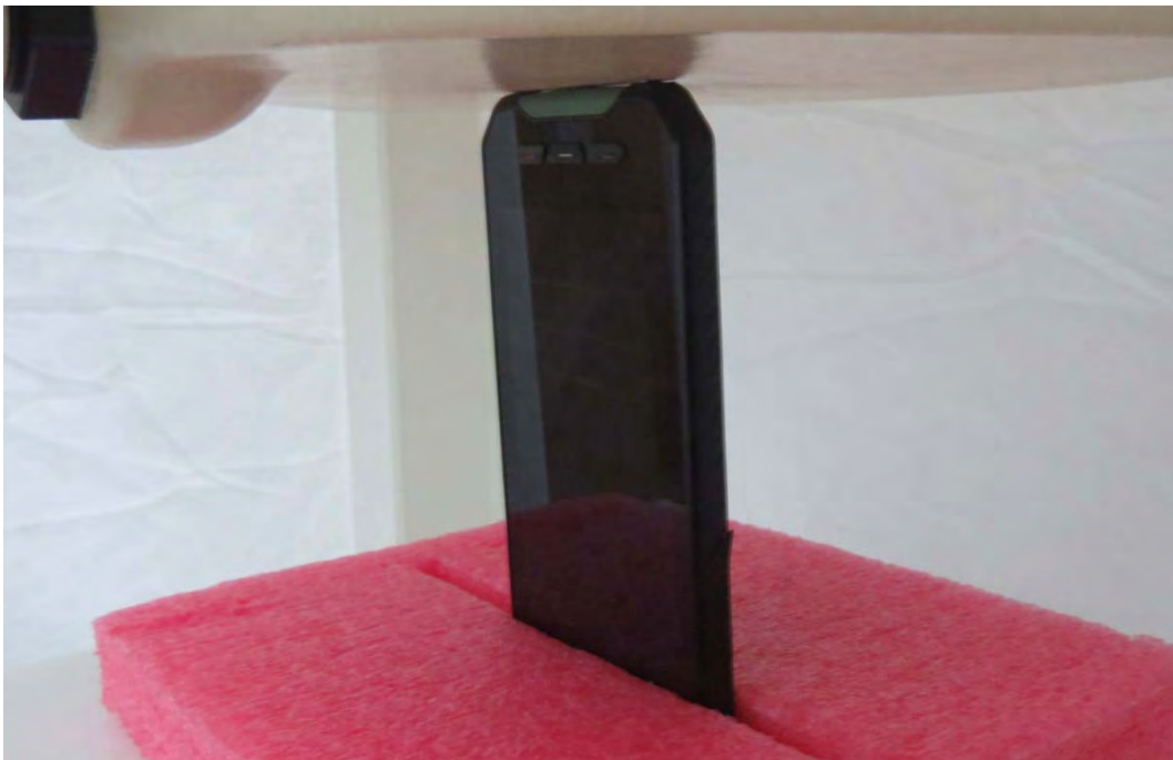
Picture 23: Bottom Side, the distance from handset to the bottom of the Phantom is 0mm
