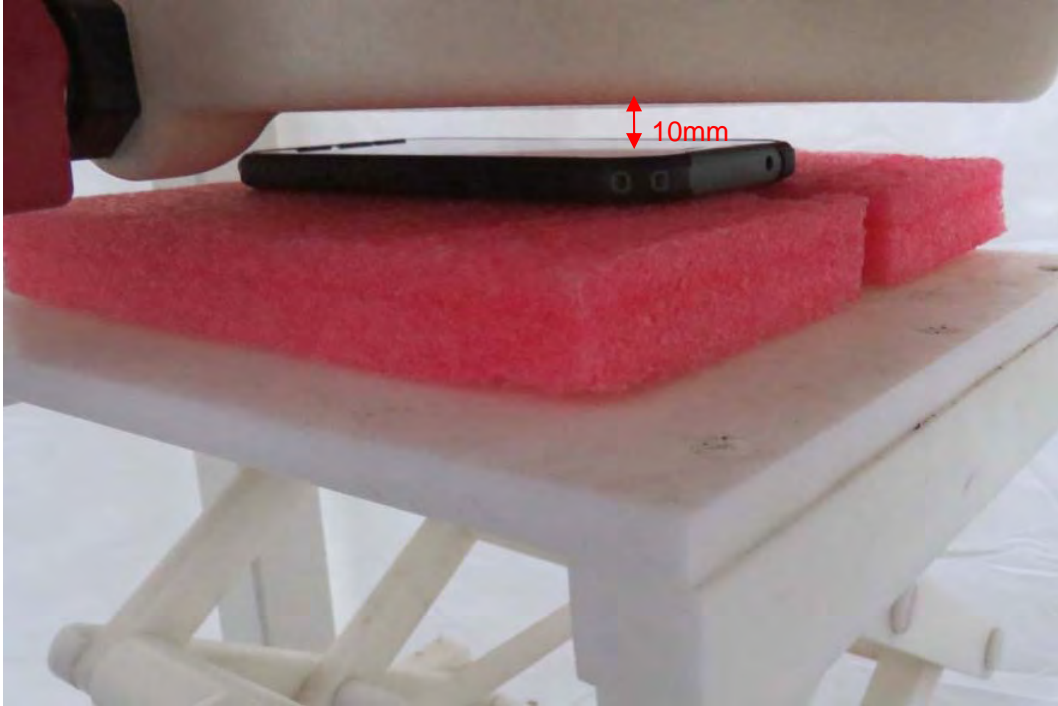
Picture 12: Front Side, the distance from handset to the bottom of the Phantom is 10mm
