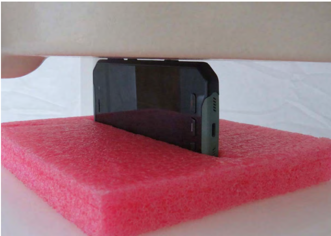
Picture 21: Right Side, the distance from handset to the bottom of the Phantom is 0mm
