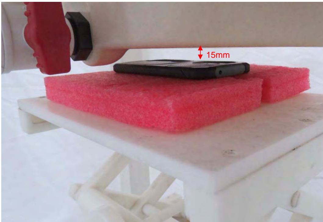
Picture 11: Back Side, the distance from handset to the bottom of the Phantom is 15mm
