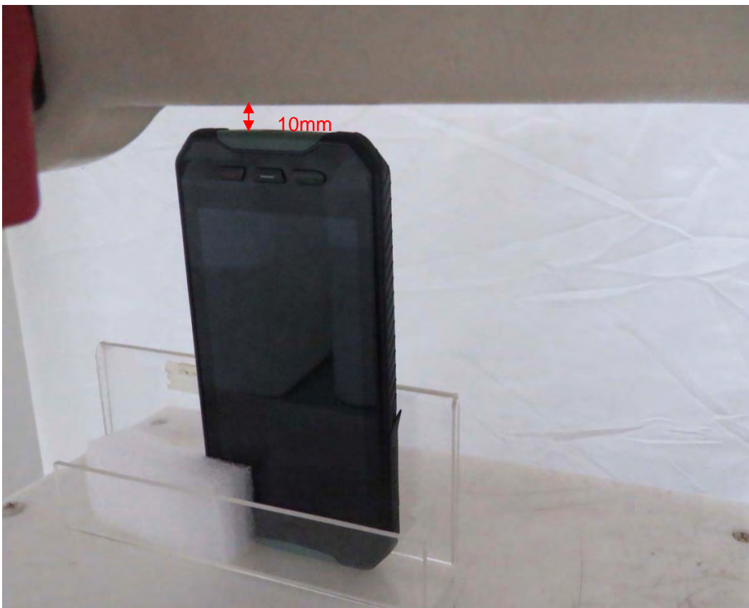
Picture 17: Bottom Side, the distance from handset to the bottom of the Phantom is 10mm
