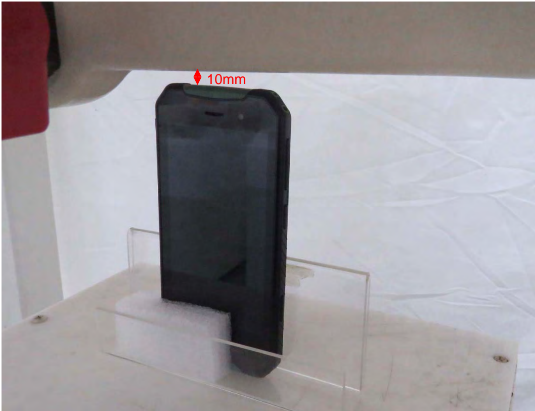
Picture 16: Top Side, the distance from handset to the bottom of the Phantom is 10mm
