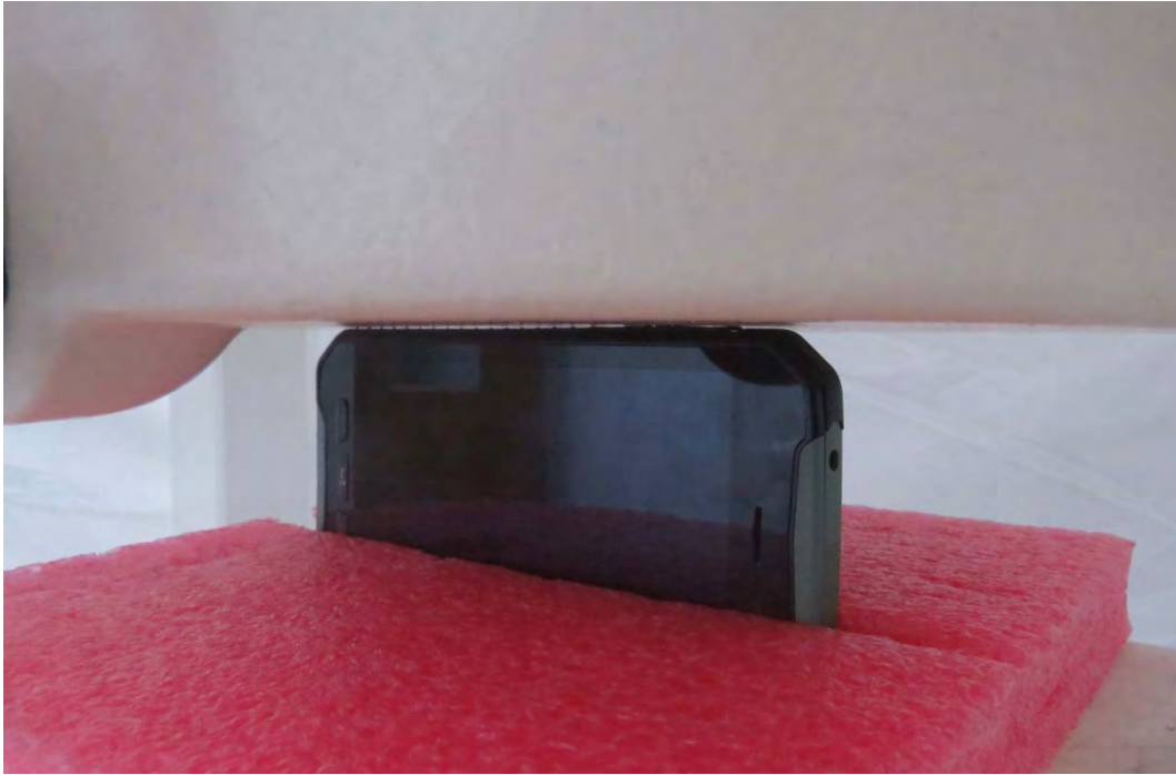
Picture 20: Left Side, the distance from handset to the bottom of the Phantom is 0mm
