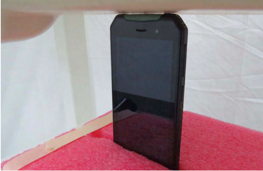
Picture 22: Top Side, the distance from handset to the bottom of the Phantom is 0mm
