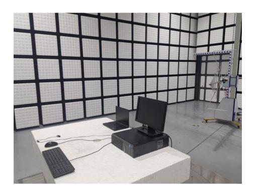
Test Mode: Mode 2 Description: Front view of Radiated Emission Test Setup (Above 1GHz)
