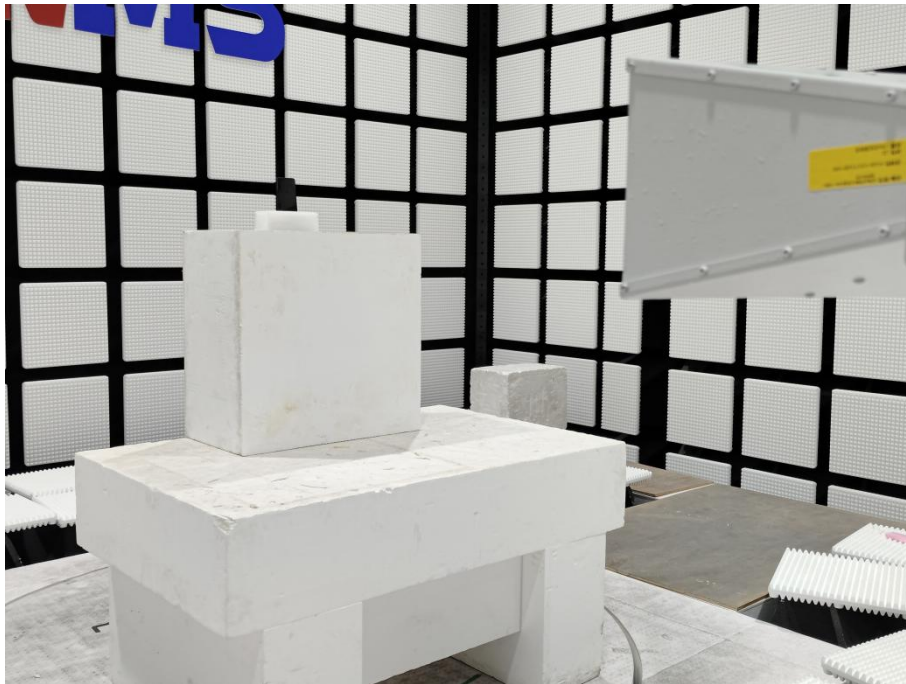
Description: Radiated Emission Test Setup (1GHz -18GHz)
