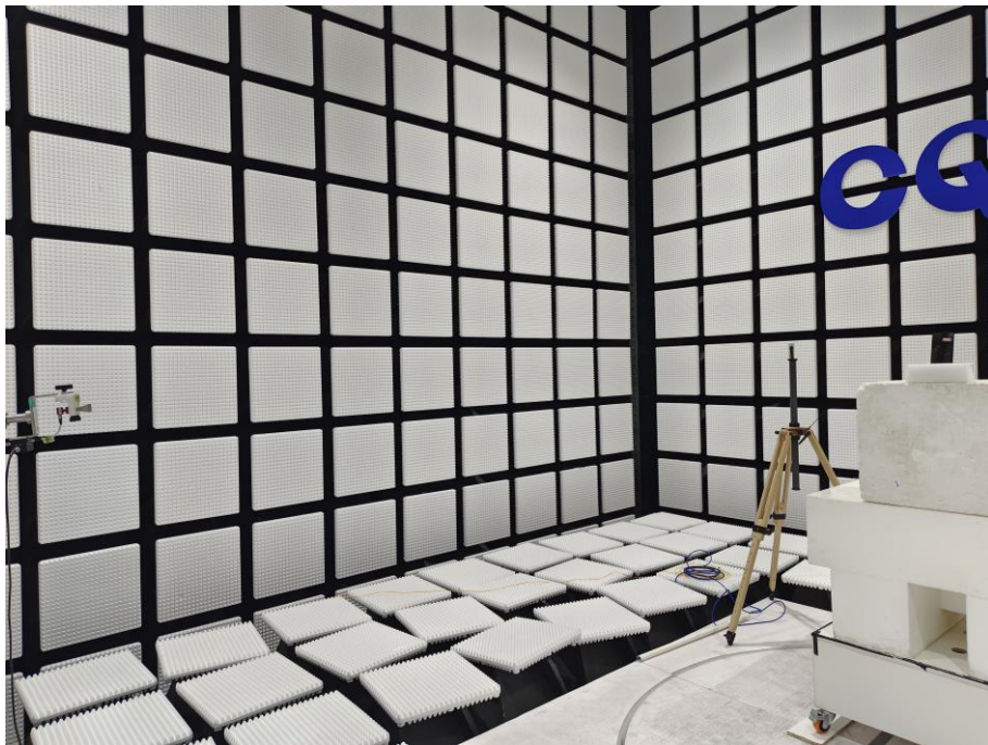
Description: Radiated Emission Test Setup (26.5GHz -40GHz)
