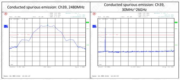
Note: 1. The out-of-limit signal in the picture is the main frequency signal.
