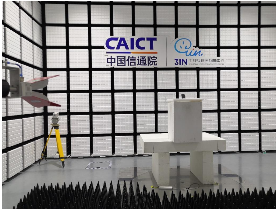
Description: Radiated Emission Test Setup (1GHz -18GHz)
