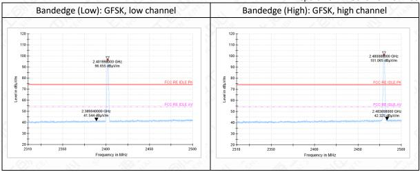
Note: The out-of-limit signal in the picture is the main frequency signal.
