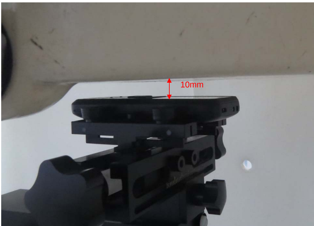
Picture 6: Front Side, the distance from handset to the bottom of the Phantom is 10mm
