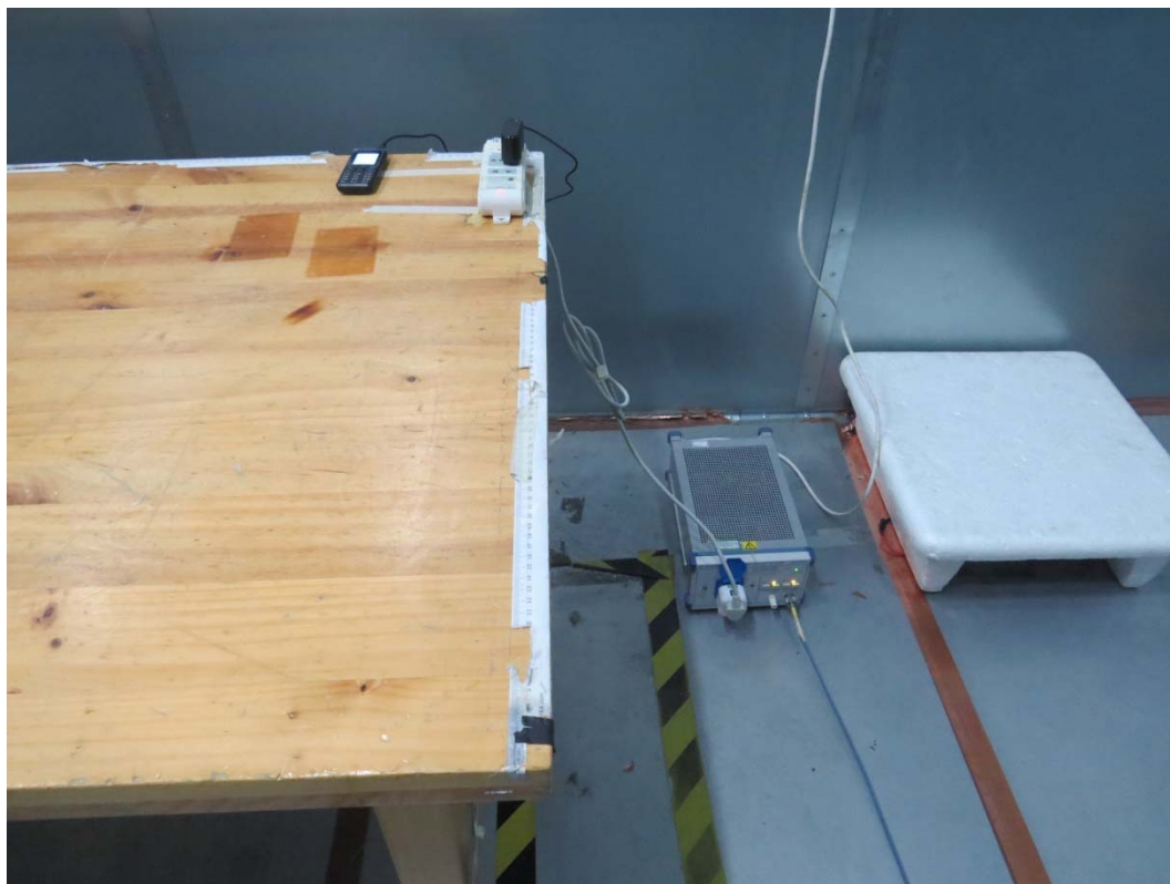
Picture 2 Conducted Emission Test Setup
