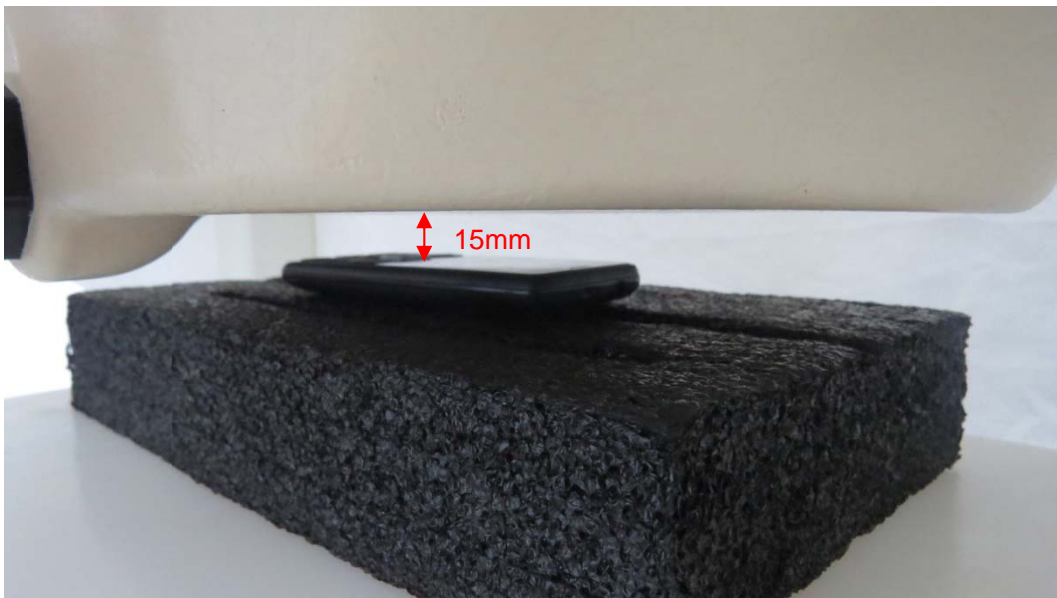
Picture 8: Front Side, the distance from handset to the bottom of the Phantom is 15mm
