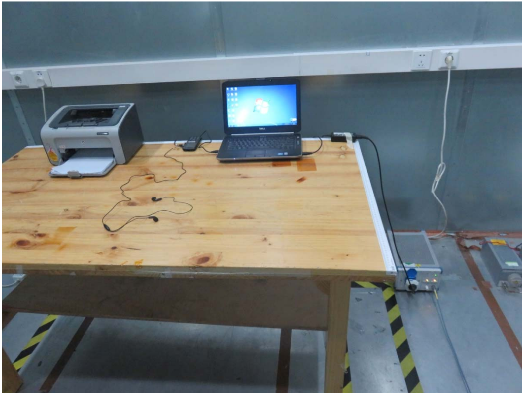
Picture 3 Conducted Emission Test Setup
