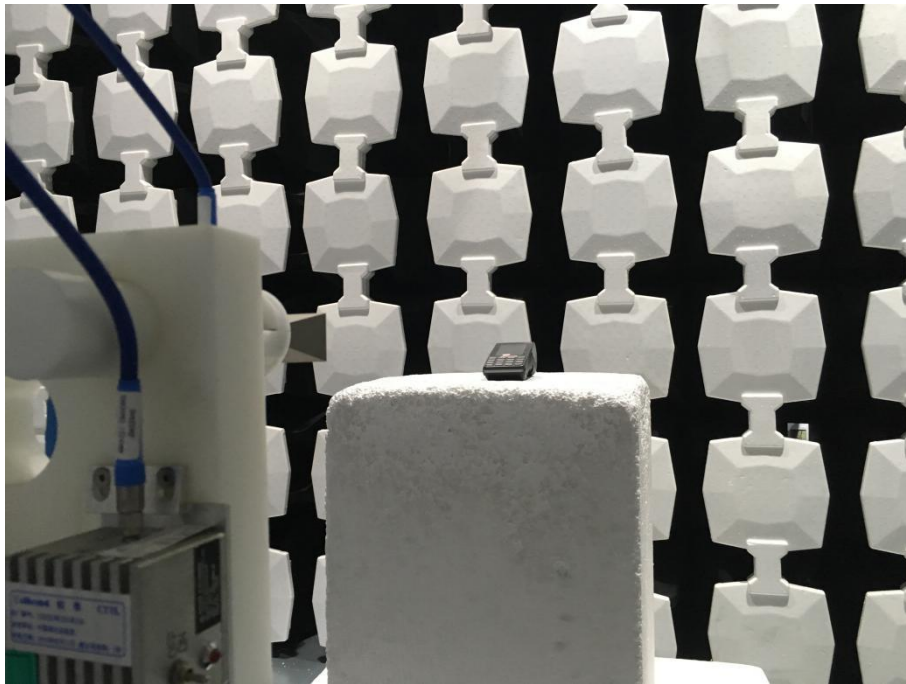
Description: Radiated Emission Test Setup (Above 18GHz)
