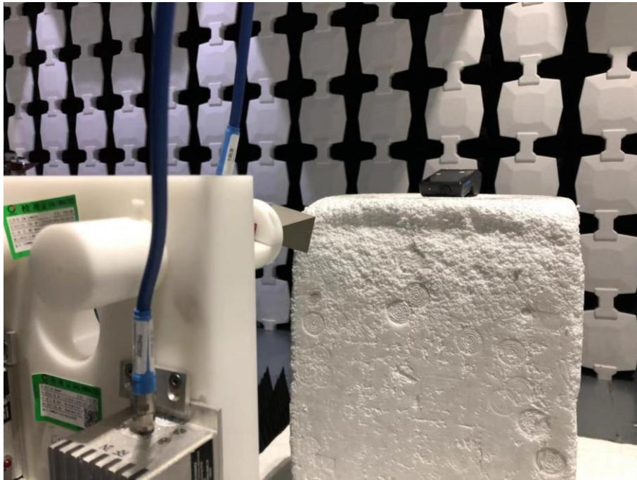
Description: Radiated Emission Test Setup (Above 18GHz)
