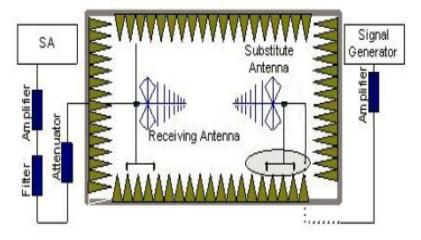
In the chamber, an substitution antenna for the frequency band of interest is placed at the reference point of the chamber. An RF Signal source for the frequency band of interest is connected to the substitution antenna with a cable that has been constructed to not interfere with the radiation pattern of the antenna. A power ( $P_{\text{Mea}}$ ) is applied to the input of the substitution antenna, and adjust the level of the signal generator output until the value of the receiver reach the
