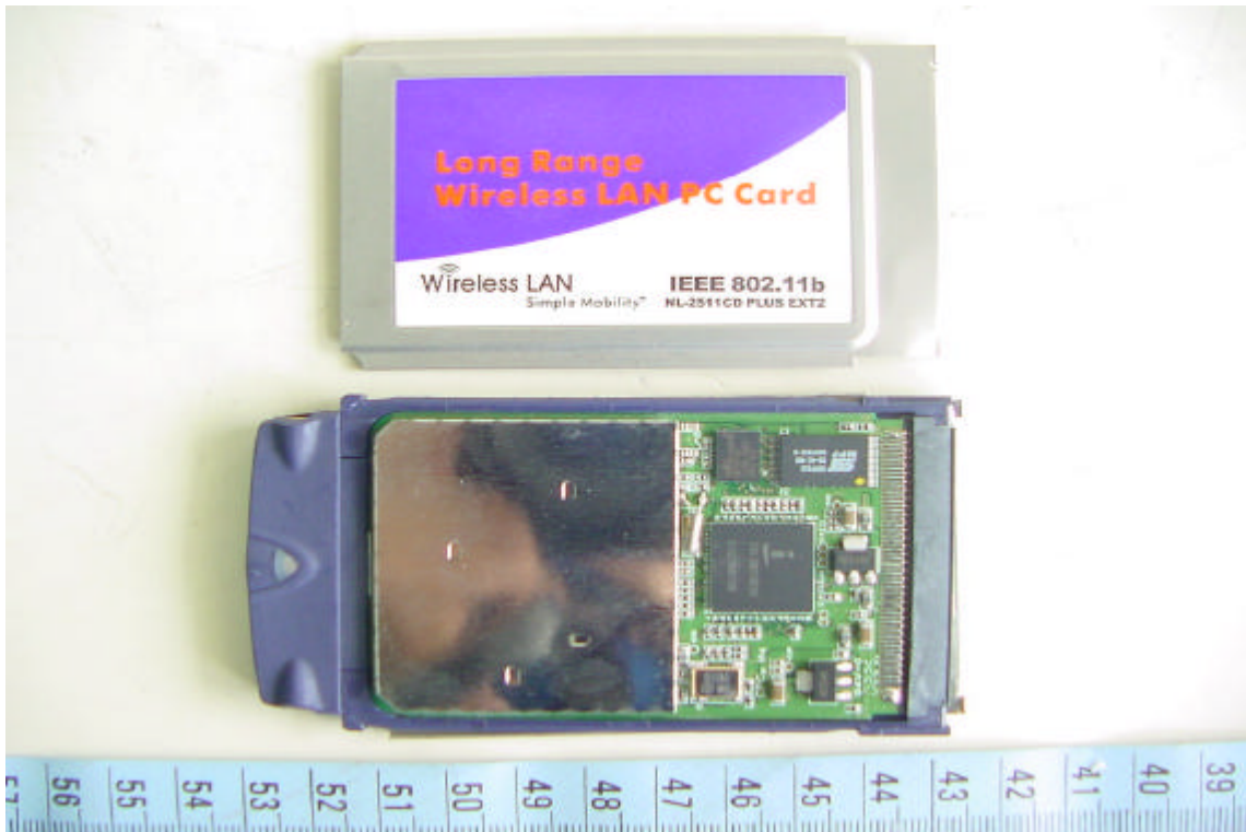
26. Internal View of RF Module
