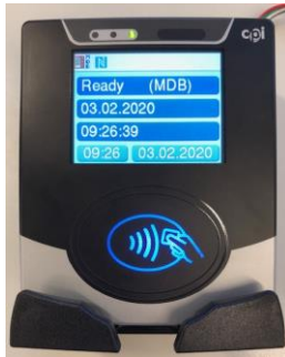
Reader ready, Connected to VMC
