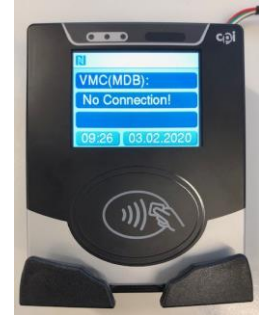
Reader not connected to VMC
