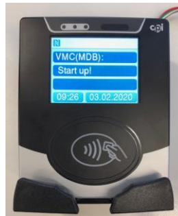
Reader starting up connection to VMC
