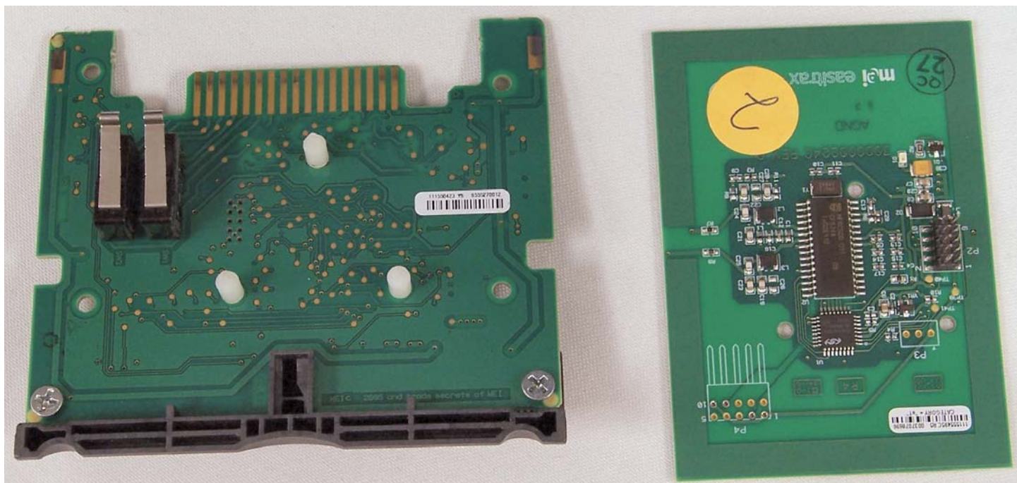
Radio Card Removed From Parent Board
