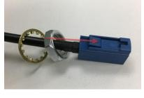
5b. Insert the locking tab into the connector and press the tab down, to lock the cable in place.
