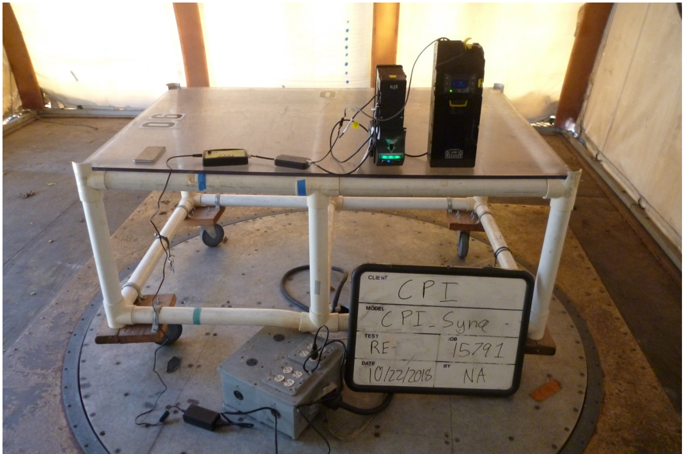
Photograph 5: Radiated Emissions Test Setup
