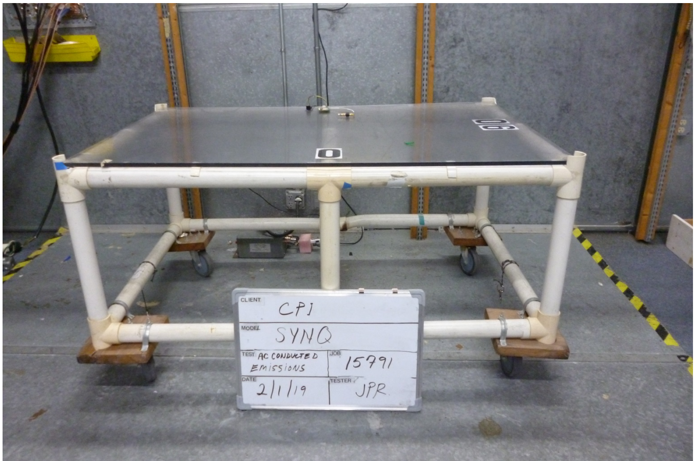
Photograph 3: Conducted Emissions Test Configuration - Front
