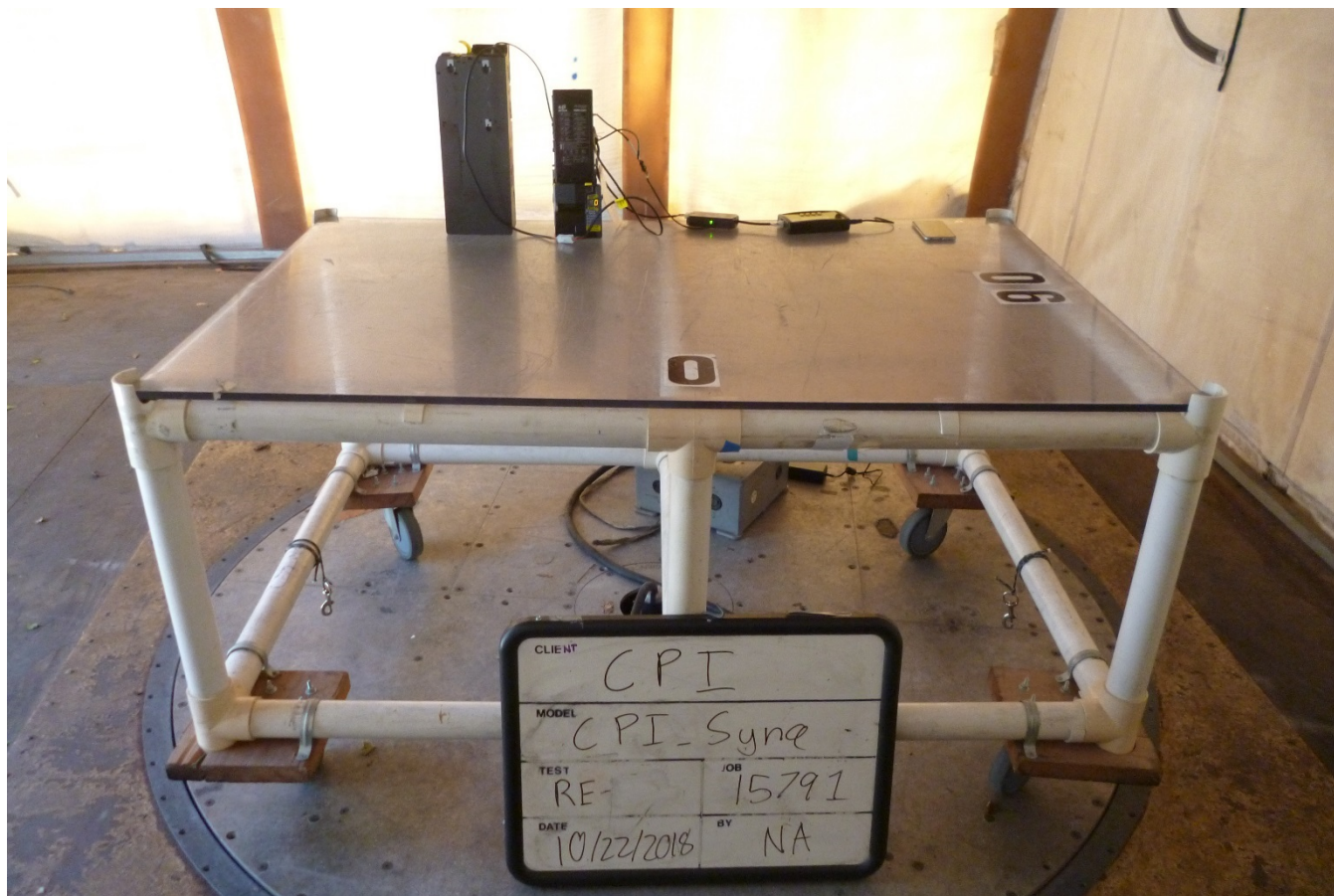
Photograph 6: Radiated Emissions Test Setup
