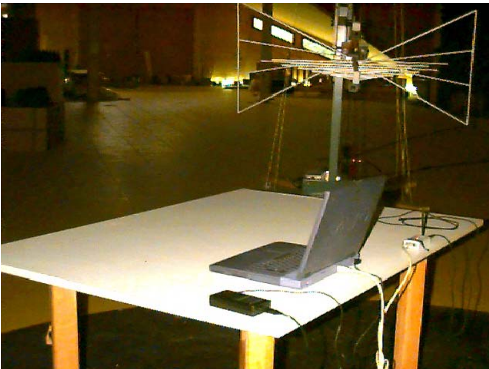
EUT supplied via USB port from SONY PCG-F403VAIO with AC Adapter PCGA-ACX1
