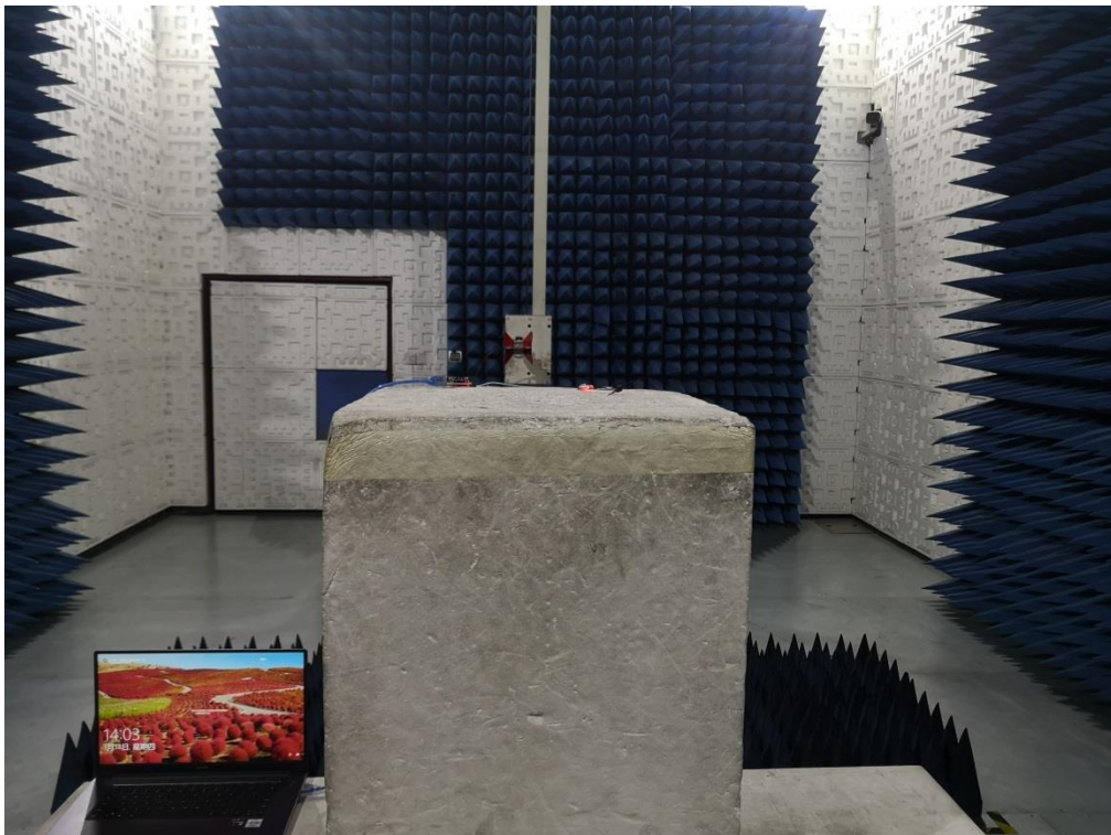
RADIATED EMISSION TEST SETUP ABOVE 1GHz
