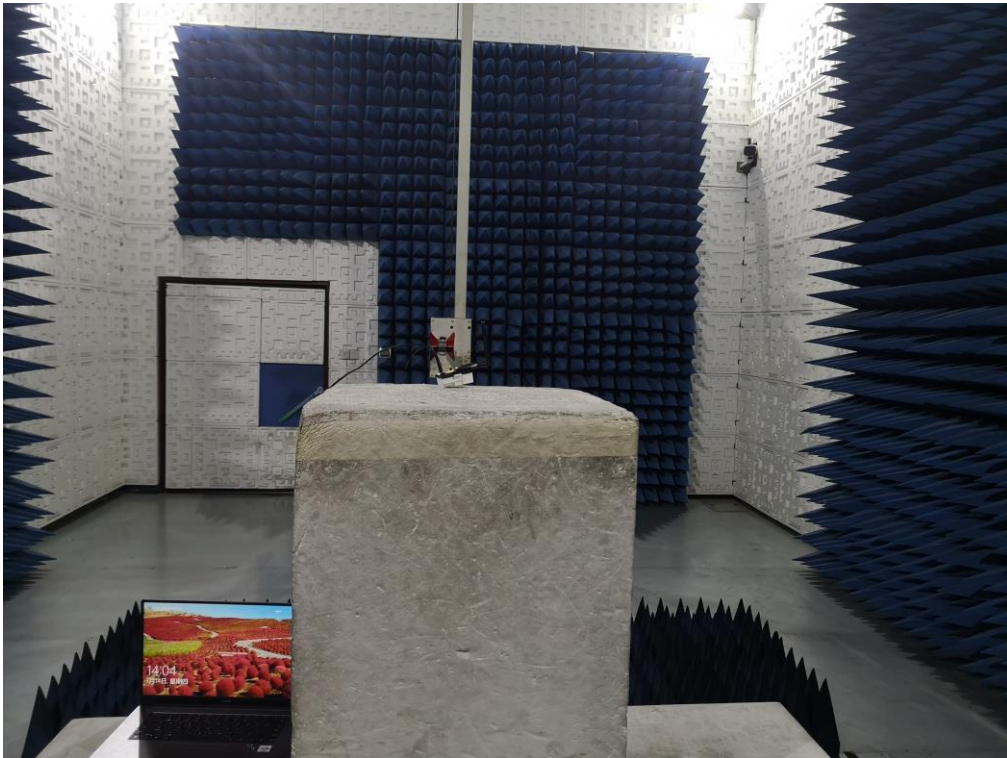
FCC RADIATED EMISSION TEST SETUP ABOVE 1GHZ
