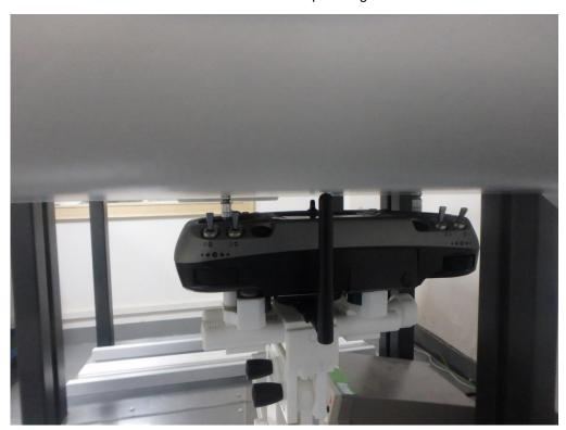
Edge2- Rotate the antenna up 90 degrees 0mm
