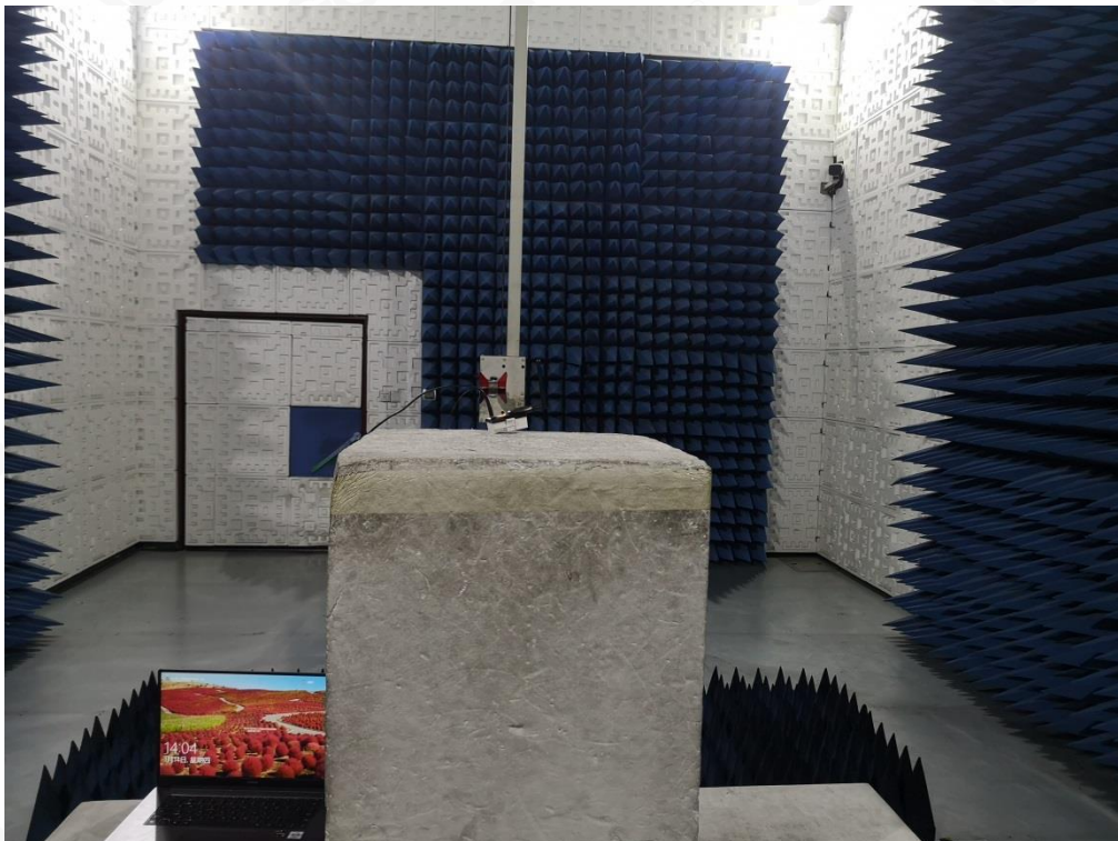
FCC RADIATED EMISSION TEST SETUP ABOVE 1GHZ
