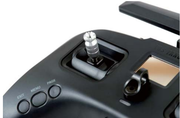
Left gimbal and configuration menu buttons
