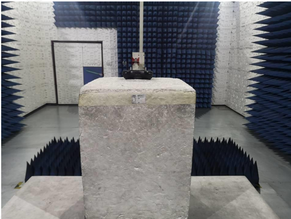
FCC RADIATED EMISSION TEST SETUP ABOVE 1GHZ
