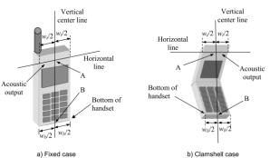
3. Position the handset close to the surface of the phantom such that point A is on the (virtual) extension of the line passing through points RE and LE on the phantom. The plane defined by the vertical centerline and the horizontal line of the handset is parallel to the sagittal plane of the phantom
