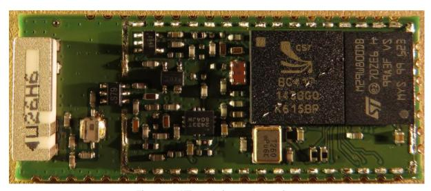
Figure 3: WT41u-A, internal, top view
