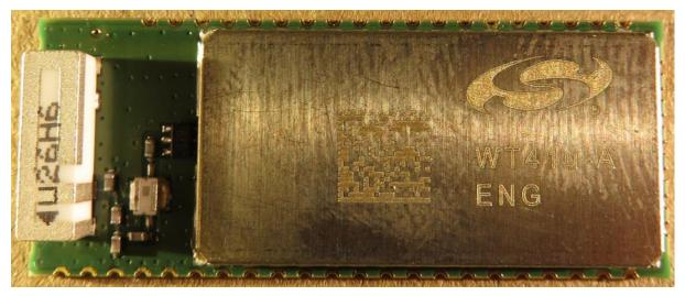
Figure 2: WT41u-A, external, top view
