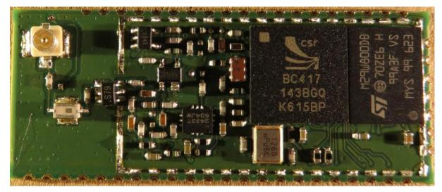
Figure 4: WT41u-E, internal, top view
