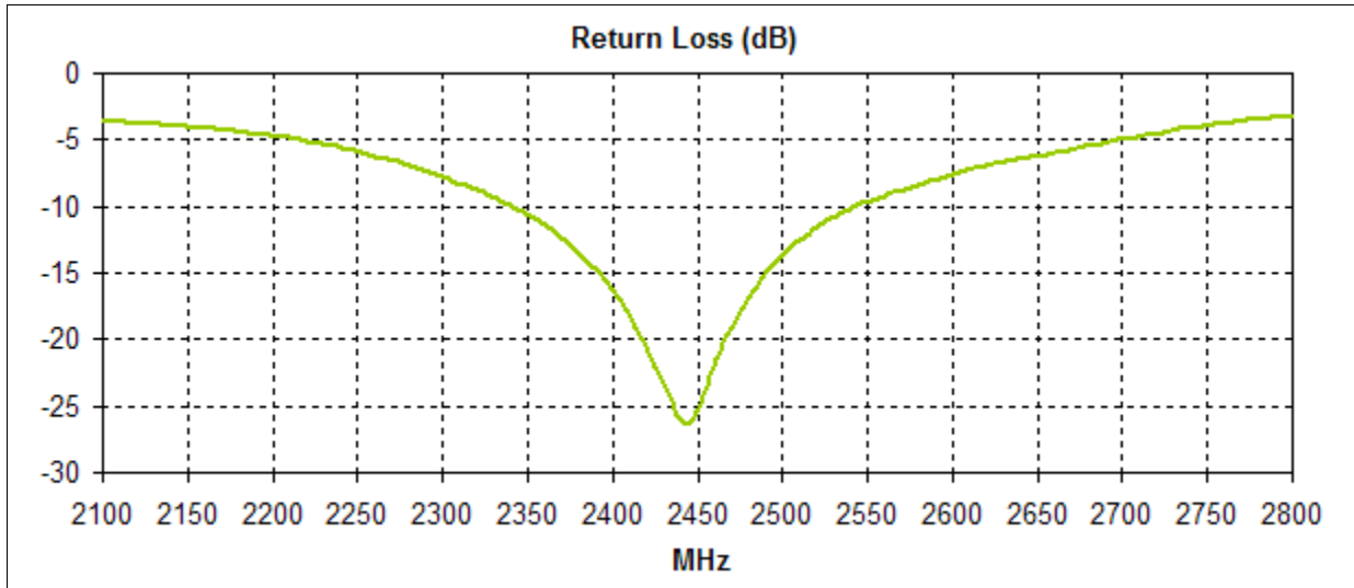
Figure 3. Return Loss for the FXP70 Antenna.
