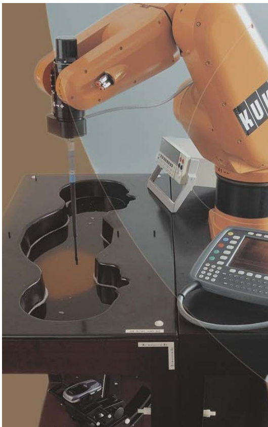
Picture A - SAR Dosimetric Assessment System
