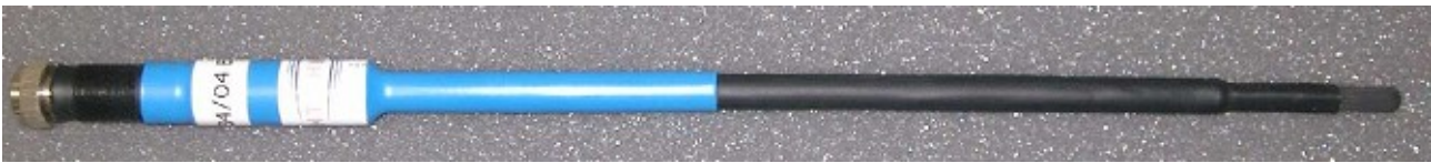
Picture D – isotropic E-Field Probe
