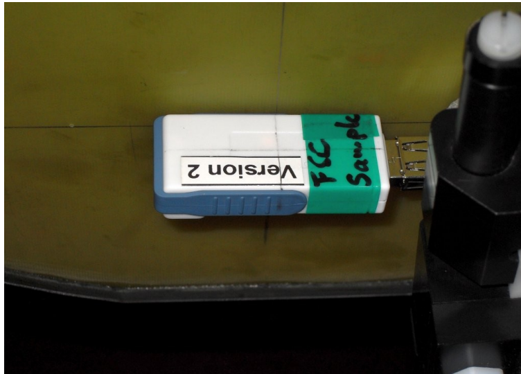
Picture 3 – Tested Device during the test USB position (C) Vertical-Front
