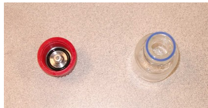
Picture F: open coaxial probe with the bottle cap
