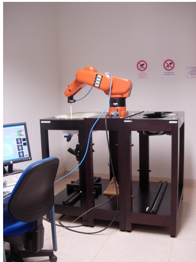
Picture A - SAR Dosimetric Assessment System
