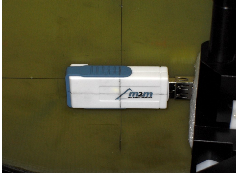
Picture 1 – Tested Device during the test USB position (A) Horizontal-Up
