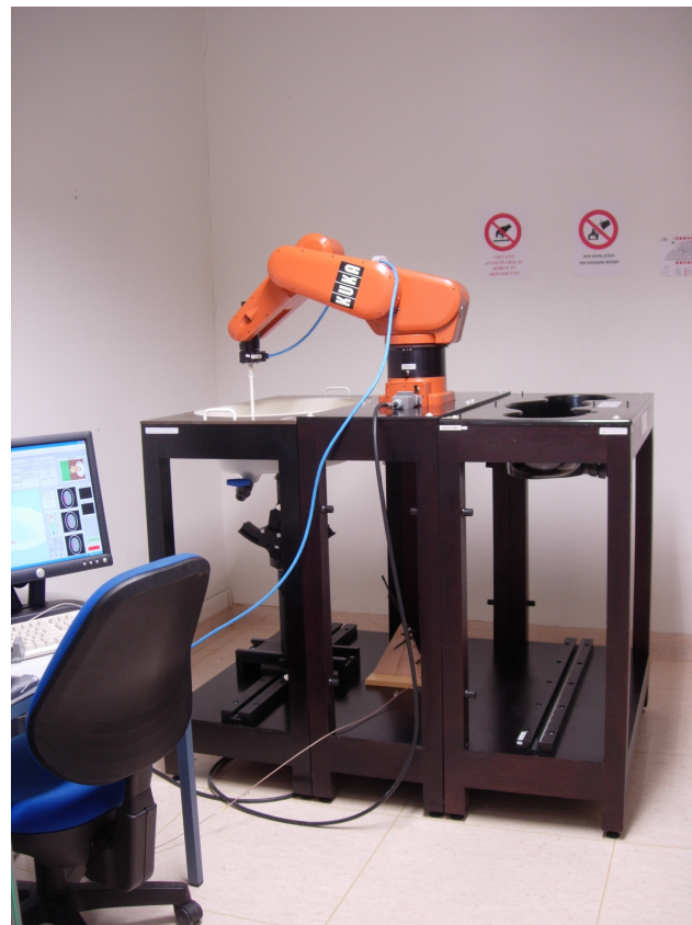
Picture A - SAR Dosimetric Assessment System
